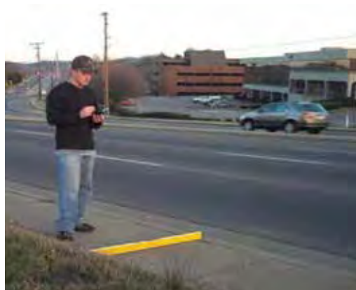
According to ADA guidelines, the maximum acceptable cross slope for a sidewalk is 2% grade.
