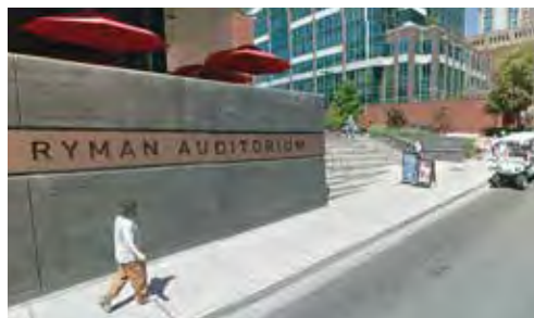
The sidewalk outside the Ryman Auditorium is 8 feet wide, greater than the 5 feet minimum standard
